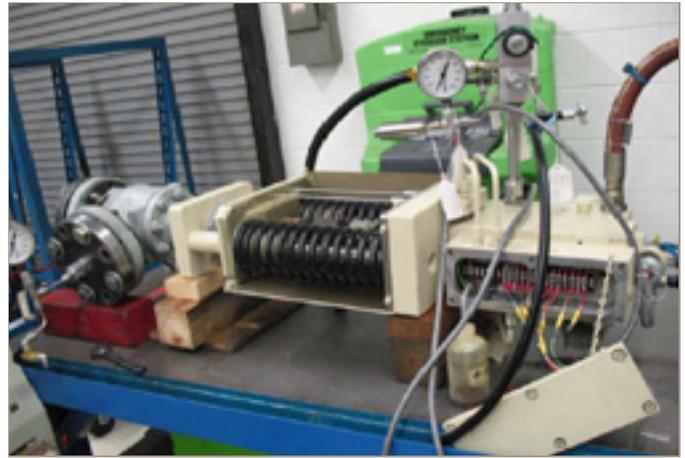
**Gas Valve Actuator enduring life-cycle testing**
