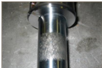
**Figure 1. Problem point: scoring between the rod and floating metal seal.**
