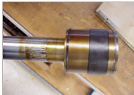
**Figure 2. Problem point: As lube oil breaks down varnish forms which is detrimental to servo actuator operation.**
