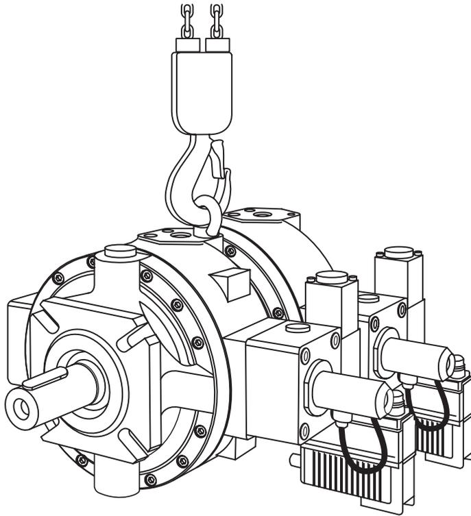
Fig. 18: Transporting Multiple Pumps with Lifting Tackle
