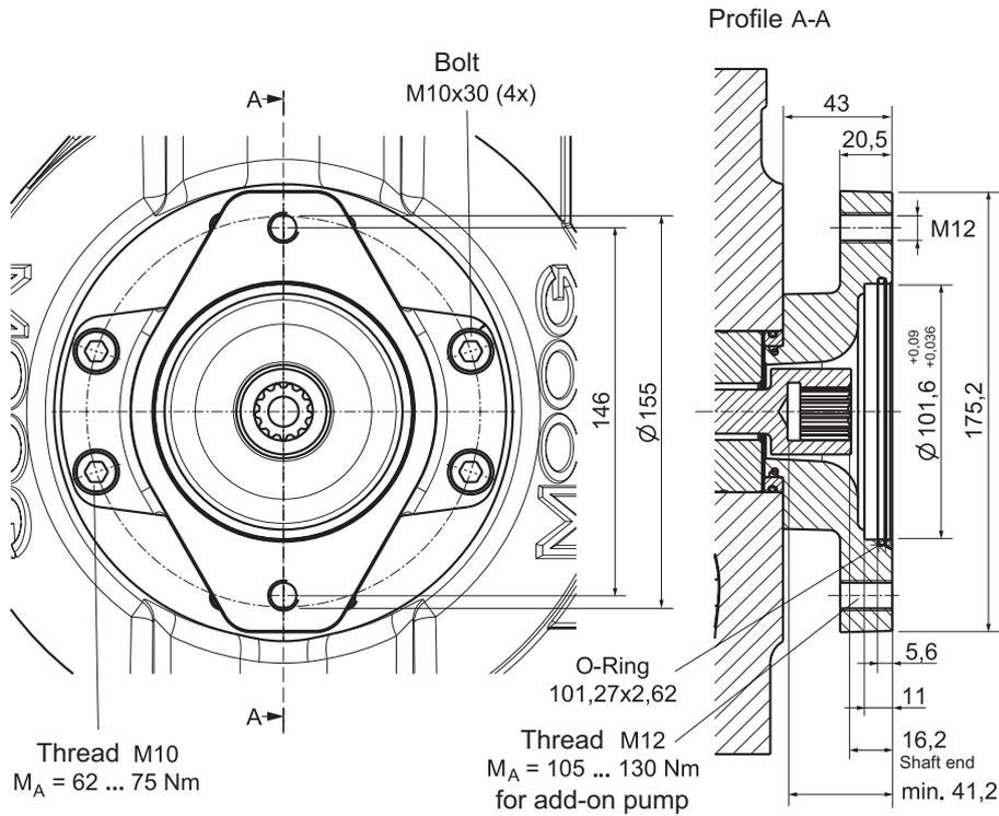
Fig. 23: Adapter flange SAE-B with 13-tooth shaft
