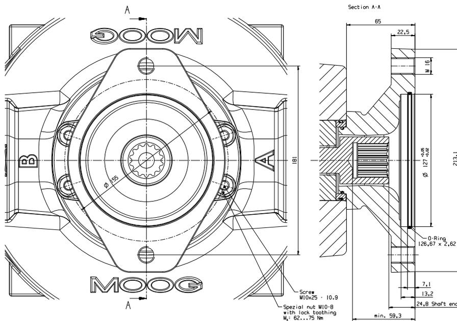
Fig. 24: Adapter flange SAE-C with 14-tooth shaft
