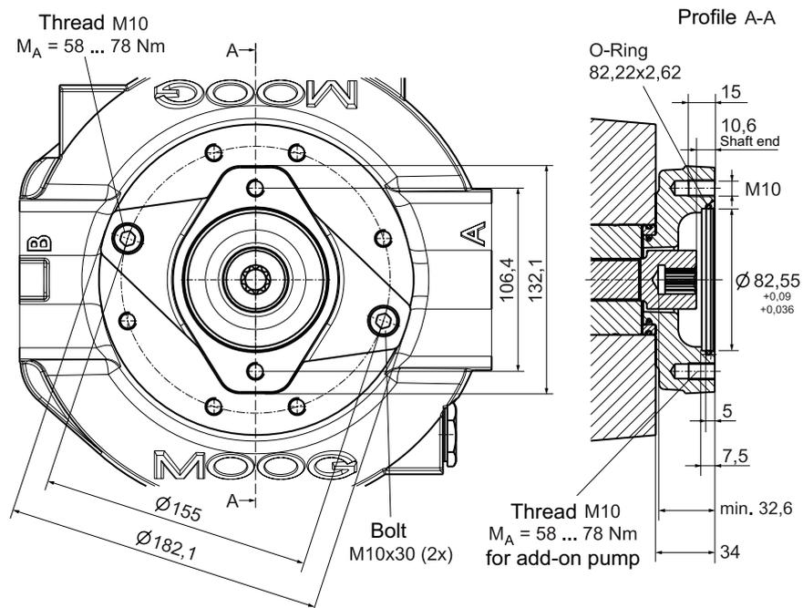
Fig. 22: Adapter flange SAE-A with 9-tooth shaft
