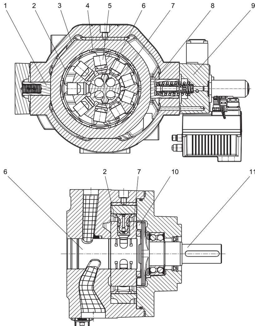
Fig. 4: Cross Section Radial Piston Pump RKP-II
